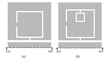
Fig. 4. Layout of the short circuits configuration for (a) M-DGS resonator and (b) CM-DGS resonator (half symmetrical view).
