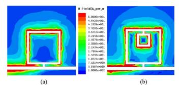
Fig. 3. Magnetic field distribution of (a) the M-DGS resonator at 2.7 GHz and (b) the CM-DGS resonator at 2.3 GHz.
