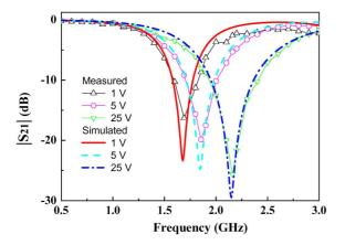
Fig. 7. Simulated and measured transmission coefficients for the tunable bandstop resonator.
