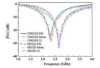
Fig. 2. Electromagnetic (EM) and circuit (Ct) simulated and measured transmission coefficients for the M-DGS and CM-DGS resonator.
