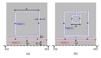
Fig. 1. Schematic diagram of (a) M-DGS resonator and (b) proposed compact M-DGS resonator (half symmetrical view).
